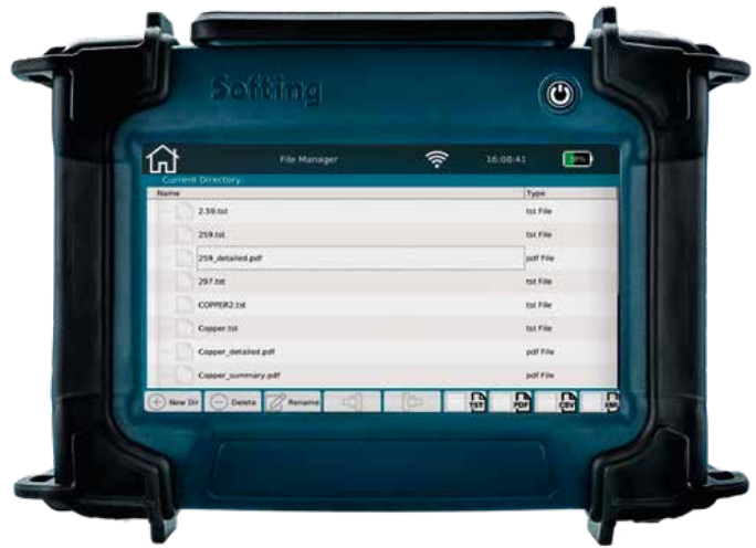
The file manager can be accessed directly from the home screen. NetXpert XG generates detailed result reports in PDF or CSV format
