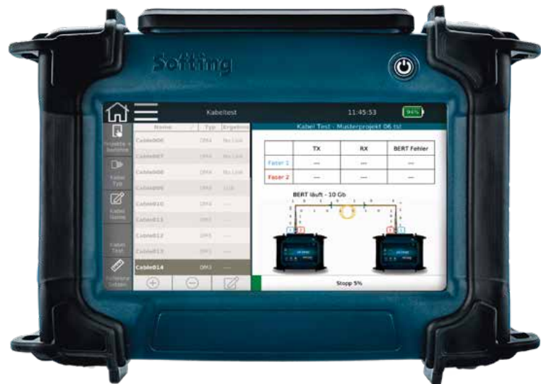
Standards-compliant signal-to-noise ratio and bit error rate tests (BERT) show the performance limits of cabling, both copper and fiber optic (BERT only) (shown here)
